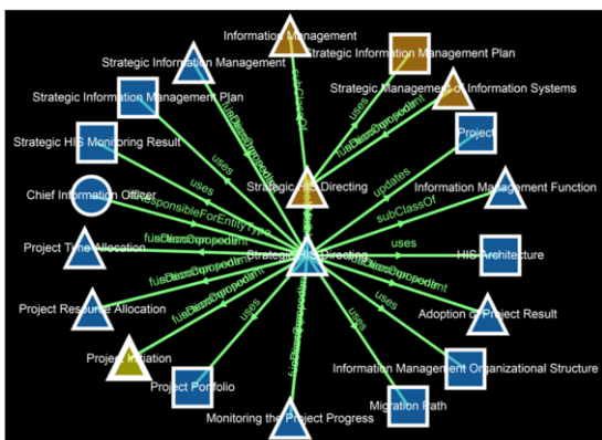
Figure 2 - Circle star for the function “Strategic HIS Directing” (rectangles represent entity types, triangles represent functions and circles represent roles).
